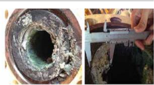
Section 8: ID = 126mm ( Otiginal ID=199 mm), Scale thickness T max = 50mm, T min = 25mm
