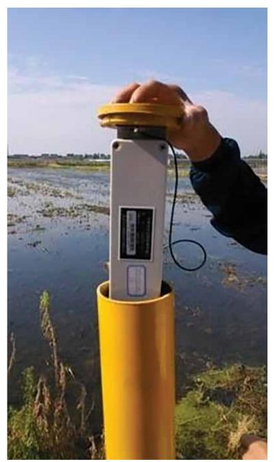
Figure 9. Intelligent data sampling units installed in test posts along the pipeline.
