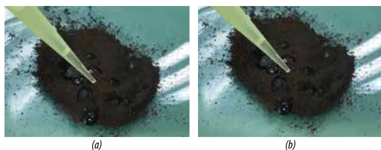
Figure 4. Image of water droplet on Fe_3O_4 powder before (a) and after (b) modification.
