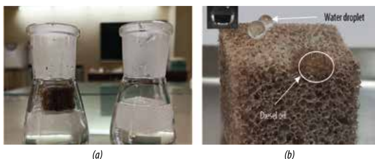
Figure 6. Photograph of sponge used to test the hydrophobic and oleophilic behavior: (a) Sponge coated with modified HDPE- Fe_3O_4 coating (64%) vs. pristine sponge on the water surface; (b) Water droplet and diesel oil droplet on the sponge coated with modified HDPE- Fe_3O_4 coating (inset shows the corresponding water contact angle).
