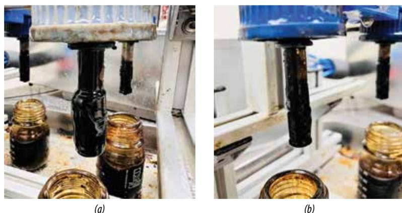
Figure 7. Wax tendency of crude oil pumped from RP-1, before (a) and after (b) optimized treatment.
