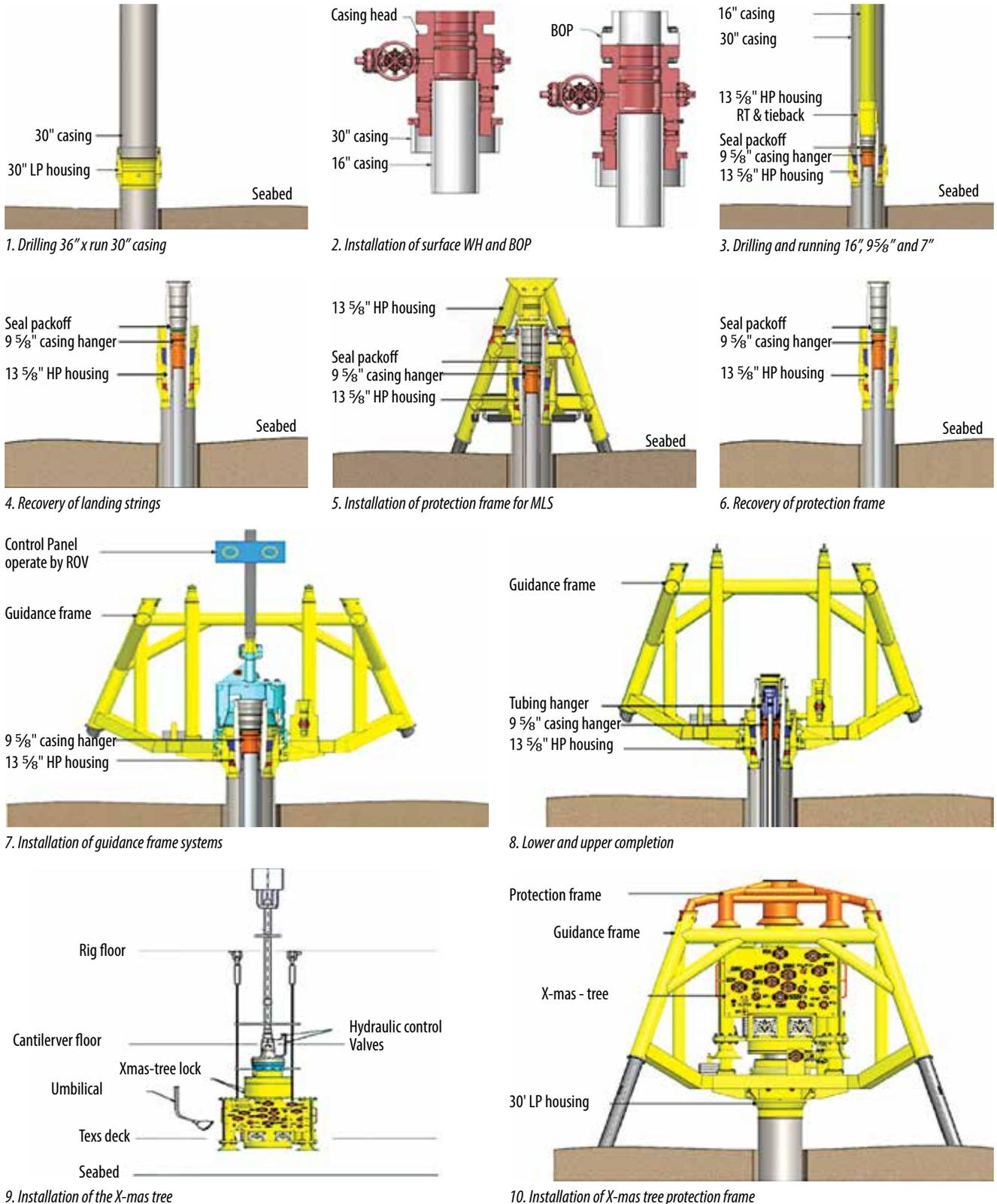
Figure 2. Running procedures of subsea wellhead and MLS systems.
