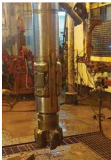
Figure 17. No bit-balling while drilling.
