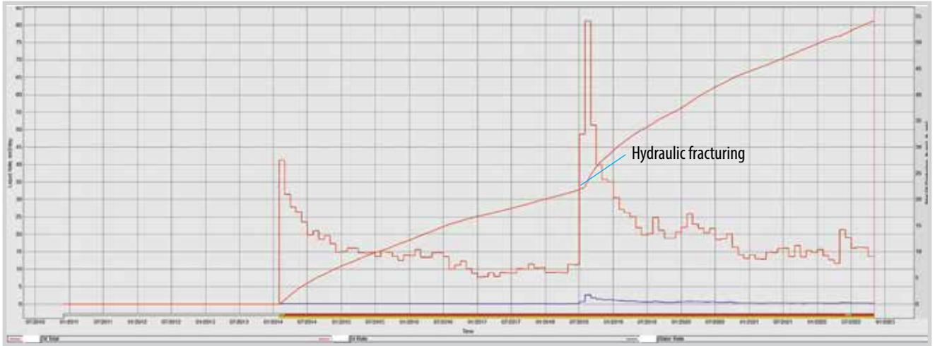
Figure 5. Production of well BO-01 before and after hydraulic fracturing.
