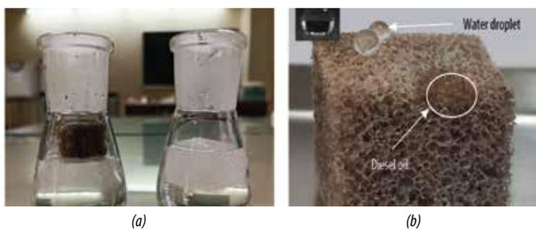
Figure 6. Photograph of sponge used to test the hydrophobic and oleophilic behavior: (a) Sponge coated with modified HDPE-Fe<sub>3</sub>O<sub>4</sub> coating (64%) vs. pristine sponge on the water surface; (b) Water droplet and diesel oil droplet on the sponge coated with modified HDPE-Fe<sub>3</sub>O<sub>4</sub> coating (inset shows the corresponding water contact angle).
