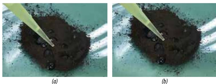
Figure 4. Image of water droplet on Fe<sub>3</sub>O<sub>4</sub> powder before (a) and after (b) modification.
